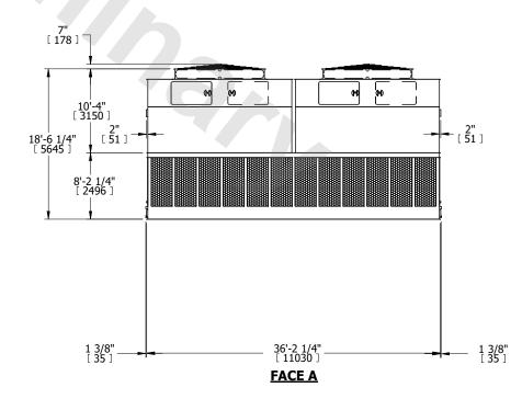
SHIPPING WEIGHT 50360 lbs+ [22845] kg+ OPERATING WEIGHT 87060 lbs+ [39490] kg+ HEAVIEST SECTION WEIGHT 8520 lbs+ [3865] kg+ NO. OF SHIPPING SECTIONS 6 DRAWN BY: KDS
