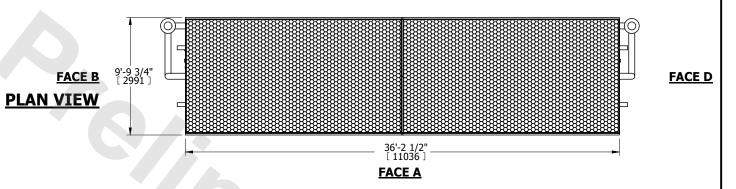
4'-9" \* [ 1448 ] (4) 4" [100] PE REFRIG IN 4'-9 5/8" [ 1464 ] (4) 4" [100] PE RÉFRIG OUT (2) ACCESS DOOR 2" [50] MPT (2) 3" [80] FPT MAKE-UP OVERFLOW 2'-7 1/2" [ 800 ] 2'-1/8" [ 613 ] 2'-7 3/4" [ 806 ] 3 5/8" [ 92 ] 3'-7 1/4" [ 1099 ] - 3" [80] MPT DRAIN 4'-1 7/8" [ 1267 ] 9'-9 3/4" —**-**FACE B
