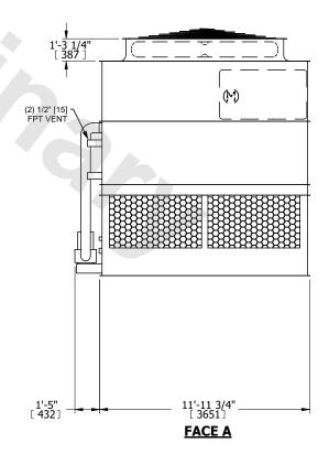
DRAWN BY: SLR NO. OF SHIPPING SECTIONS **SHIPPING** OPERATING HEAVIEST SECTION 12040 lbs+ [5465] kg+ 14590 lbs+ [6620] kg+ 22100 lbs+ [10025] kg+ WEIGHT WEIGHT WEIGHT
