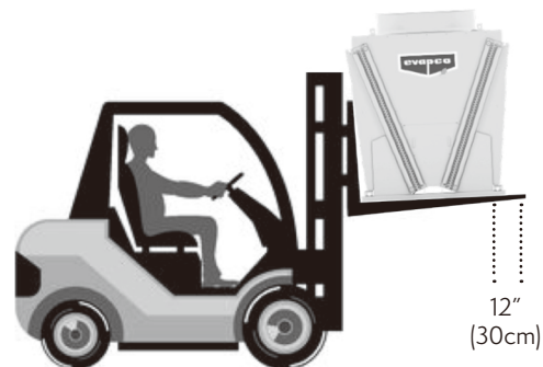
Figure 12 – V-Coil Unit Forklift Lifting Requirements
