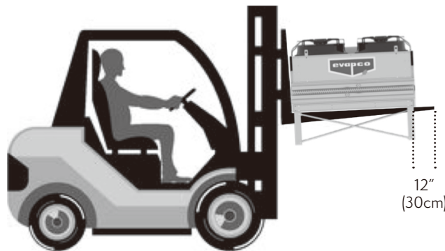
Figure 4 – Flat Coil Unit Forklift Lifting Requirements
