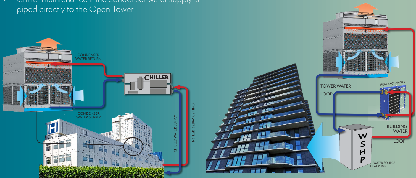
Open Loop Tower Piped to Heat Exchanger, Piped to Water Source Heat Pump
