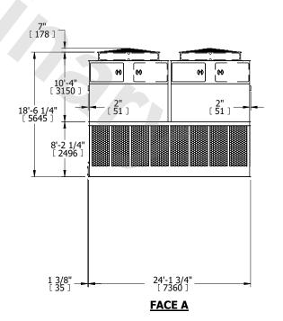
DRAWN BY: JLG NO. OF SHIPPING SECTIONS **SHIPPING** OPERATING HEAVIEST SECTION 36500 lbs+ [16560] kg+ 60820 lbs+ [27590] kg+ 6230 lbs+ [2830] kg+ WEIGHT WEIGHT WEIGHT
