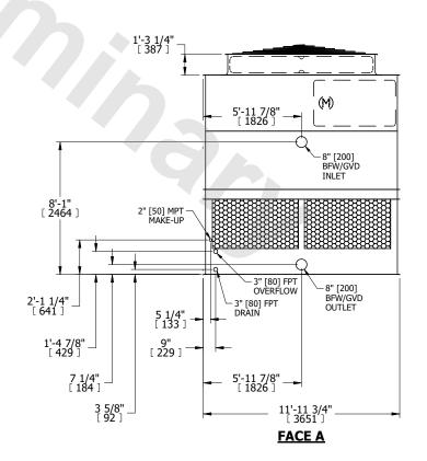
SHIPPING WEIGHT 6740 lbs+ [3060] kg+ OPERATING WEIGHT 11700 lbs+ [5310] kg+ HEAVIEST SECTION WEIGHT 4320 lbs+ [1960] kg+ NO. OF SHIPPING SECTIONS 2 DRAWN BY: JLG
