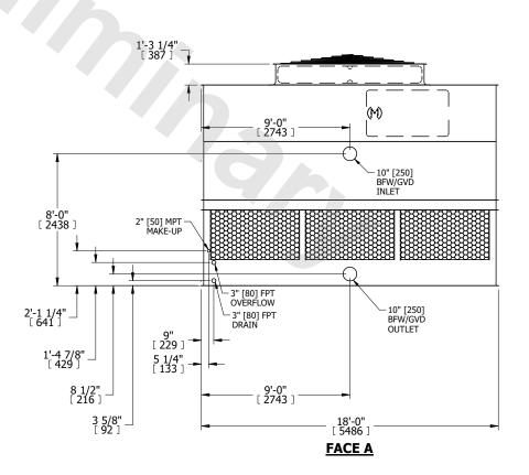
SHIPPING WEIGHT 9260 lbs+ [4205] kg+ OPERATING WEIGHT 16860 lbs+ [7650] kg+ HEAVIEST SECTION WEIGHT 5710 lbs+ [2595] kg+ NO. OF SHIPPING SECTIONS 2 DRAWN BY: KDS
