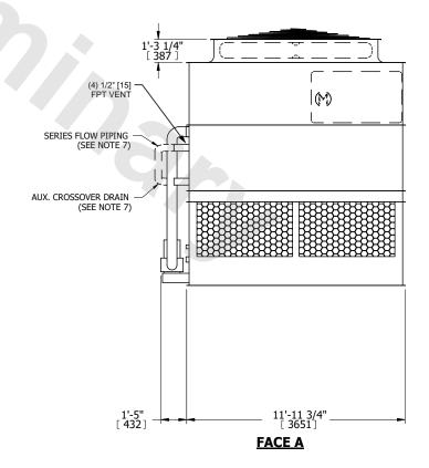
DRAWN BY: NO. OF SHIPPING SECTIONS **SHIPPING** OPERATING HEAVIEST SECTION 12040 lbs+ [5465] kg+ 14590 lbs+ [6620] kg+ 22100 lbs+ [10025] kg+ WEIGHT WEIGHT WEIGHT
